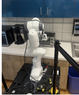
Figure 6: Real-Robot Platform. Our real-world setup features a Panda robot arm in a real kitchen.
