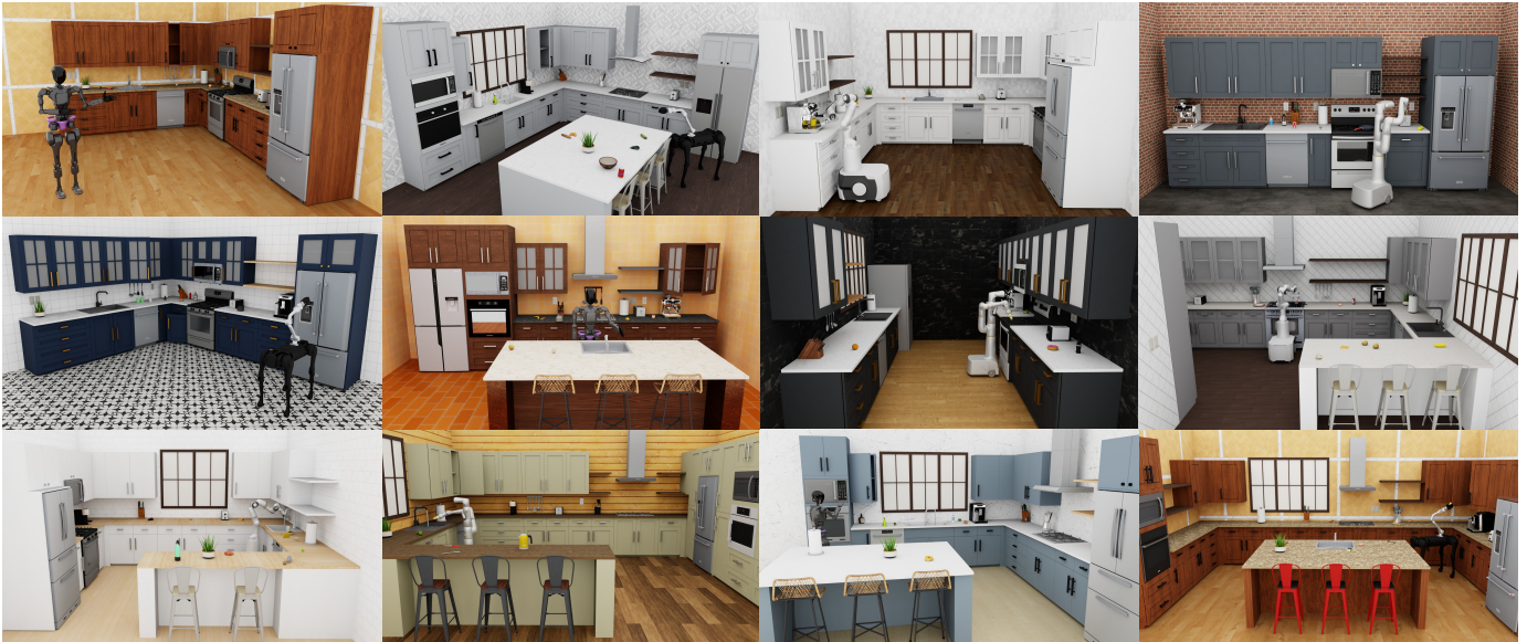
Fig. 1: Overview of RoboCasa. RoboCasa is a simulation framework for training generalist robot agents. Four pillars underlie RoboCasa: (1) Diverse assets, including 120 kitchen scenes and 2,500+ 3D objects, created with the aid of generative AI tools; (2) Cross-embodiment support for mobile manipulators and humanoid robots; (3) Diverse tasks created with the guidance of large language models; (4) Massive training datasets with over 100K trajectories.
