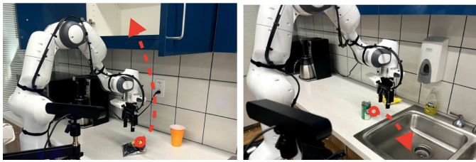
Fig. 9: Real-World Experiment Setup. We conduct experiments in a real-world kitchen environment with a Franka Emika Panda arm on a wheeled mobile platform. The two pictures illustrate two of the three evaluation tasks: (left) pick and place an object from the counter to the cabinet, and (right) pick and place an object from the counter to the sink.
